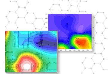
This dust migration map shows the extent of a known primary dust source (lower center) and identified an unknown secondary source in a welding cell (upper left).
